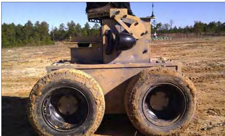
Smart targets can run five-minute miles and withstand 7.62 mm machine gun fire. [Photo courtesy of Marathon Targets]
